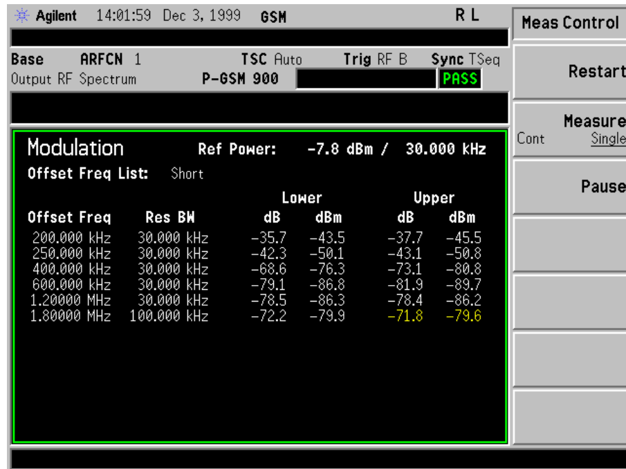
Figure 3-2 Output RF Spectrum (ORFS) Due To Modulation: Multiple Offset Measurement
